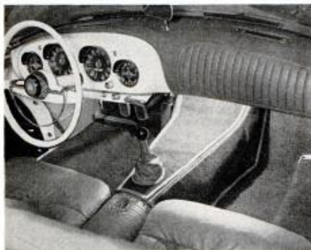
Doors on the sleek Darrin slide forward into the body. The base of the windshield is only 36 inches high
